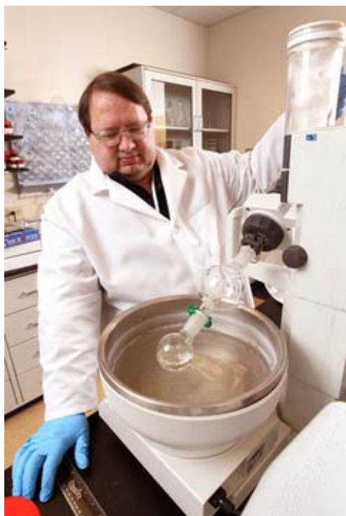
John A. Lacko | Special to the Gazette A venomous mix: Bruce Steinbaugh, of Vestaron Corp., removes solvents from a chemical reaction at the company’s laboratory in the Southwest Michigan Innovation Center in Kalamazoo. The 5-year-old company is developing new pesticides from spider venom to control insects such as worms and beetles.
